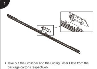
Attach the Crossbar Sliding Plate to the center of the crossbar, insert bolts (M5x12) on the side view and tighten them with the hex L – wrench (4mm). Ensure the Crossbar Sliding Plate is
